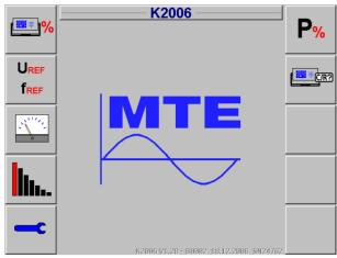
The main functions, error %, test against U-ref, f-ref, load values UI<sub>0</sub>, harmonics and basic system settings are directly accessed with soft keys.
